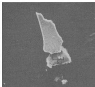
FIG. 5. (A) SEM of flat platelet in cottonseed oil mill dust and (B) EDX silicon map.
